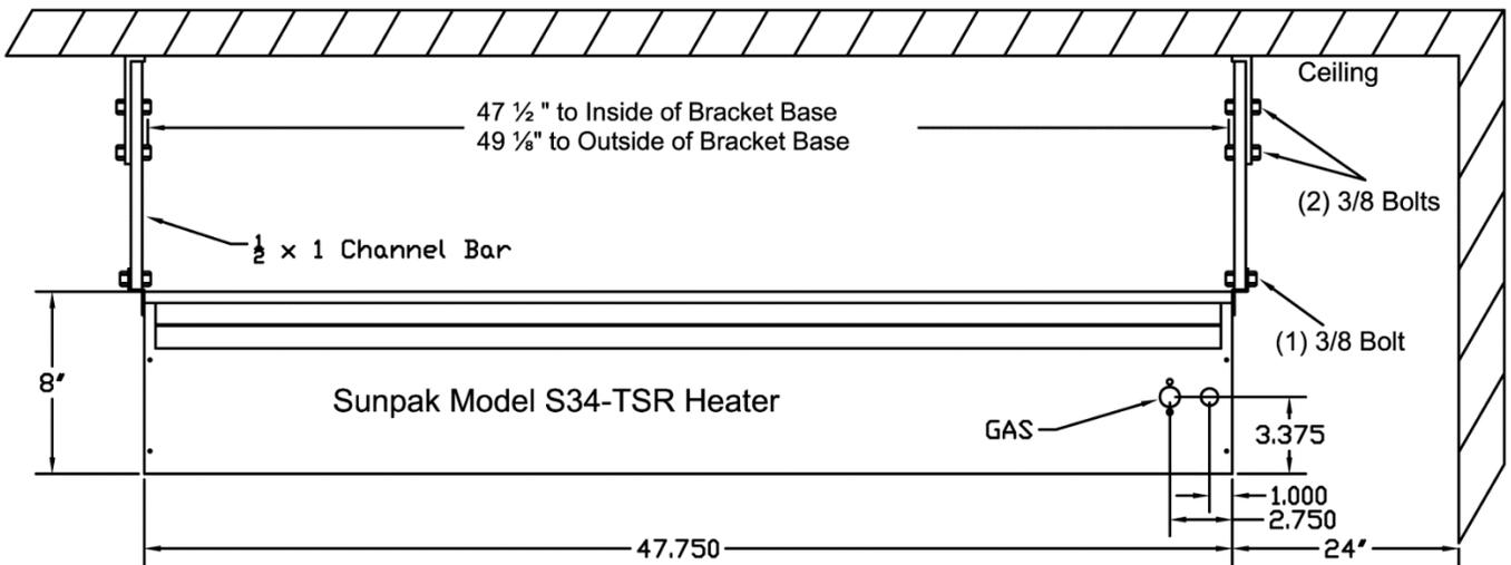
**Warning:** Heater must be level in the lengthwise direction.
