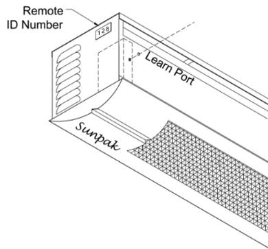
The Sunpak S34-TSR should **always** be started up and operated on the **HIGH** mode for the first 5 minutes to allow the heater to warm up. Starting up the heater on the **LOW** mode before the heater is warmed up may cause the heater to shut down prematurely. To correct this situation, press the **OFF** button followed by the **ON** button and the **HI** button. Always **PRESS** the button for at least 1 second to allow proper transmission of the remote signal.
