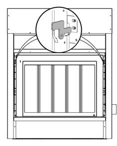
3. Ensuring the glass door is disengaged, pull the top of the door frame down and outwards to open in maintenance mode.
