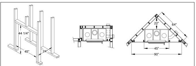
The framing dimensions are larger than required for ease of installation. Examples shown here are for a Louvered fireplace. An extra 12" is required on the left of the fireplace of a Clean Face fireplace to connect the intake air duct. The Heat Dump Option will also require an extra 12" on the selected side. Additional space, dependent on your desired installation, is also required on top and maybe on one side of the fireplace for the Central Heat Option
