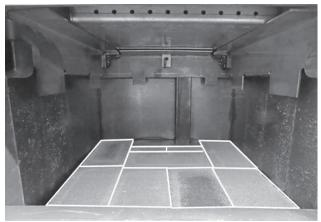
Figure 37: Floor bricks in place.
