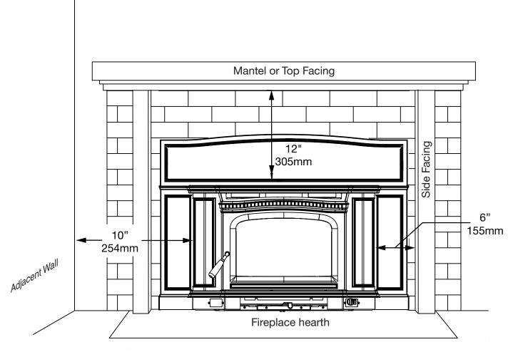
Figure 5: Clearances - ALT 5 Insert LE.
