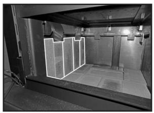
Figure 38: Left wall bricks in place.
