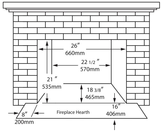
Figure 3: Fireplace opening dim. - ALT5 Insert LE.
