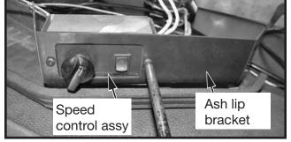
Figure 26: Relocating speed control assy and bracket.
