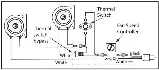
Figure 10: Wiring Diagram - Insert LE.
