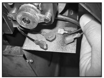
Figure 32: Disconnect the fan wires.
