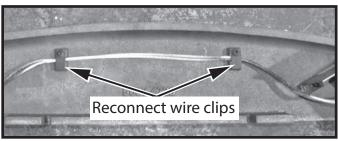
Figure 27: Reconnect wire support clips.
