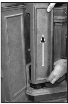
Figure 20: Fan shield removal.
