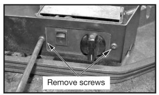
Figure 25: Speed control assy removal.
