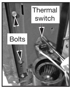
Figure 33: Remove thermal switch.
