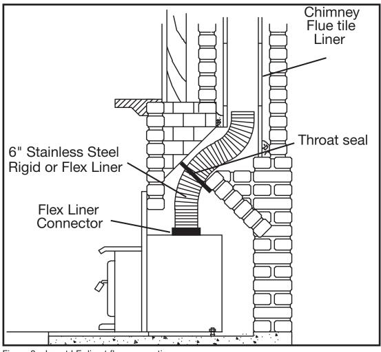
Figure 8: Insert LE direct flue connection.
