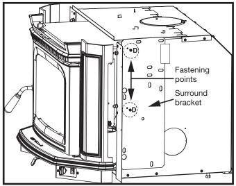
Figure 12: Removing the surround bracket.
