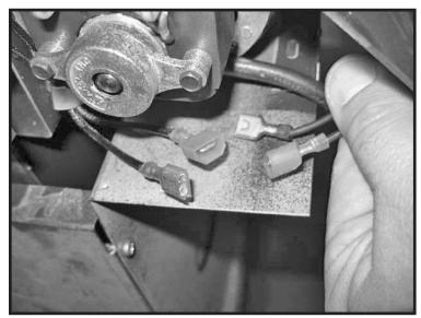
Figure 29: Reconnecting fan wires.
