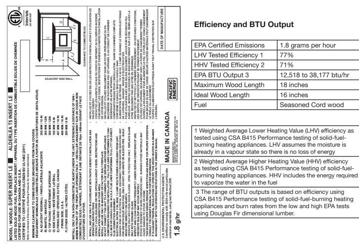
Figure 1: 100002100 - SUPER \_ ALT5 Insert LE rating Label
